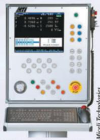
Billed as the world's fastest, the MTI CNC has a minimum processing speed of 50,000 blocks per second.
